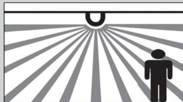
Typical mounting height for the IS 240 is 8 to 10 feet
