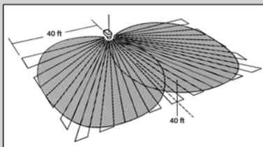
Typical mounting height for the HS 150 and HS 300 is 8 to 10 feet
