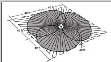
Typical mounting height for the IS 360 is 8 to 10 feet
