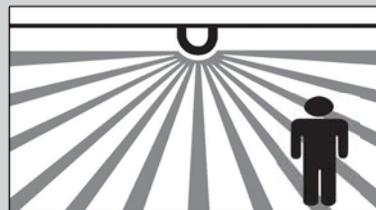
The HS 150 and HS 300's unique 180° angle of aperture enables the sensor to see straight out for greater coverage
