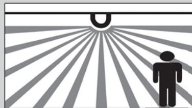
The IS 360's unique 180° angle of aperture enables the sensor to see straight out for greater coverage
